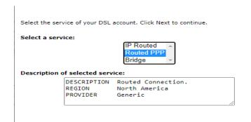
o VPI/VCI: 0/35 (Ogero), 8/35 (GDS), connections type: routed PPP over Ethernet
