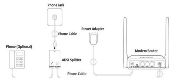
**Note:** If you have additional telephone sets, fax machine or other devices connected to the phone outlets at your premises, a splitter must be installed for each device and should be plugged into the side of the splitter that is labeled "PHONE".
